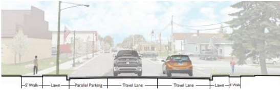
Existing Conditions Section
